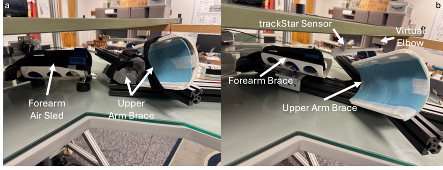
Figure 3.2. a) Natural reaching task: The participant’s upper arm was secured in a brace to restrict shoulder motion and limit movement to only elbow flexion and extension. The forearm was placed in a splint to immobilize the wrist and fingers and rested on a low-friction air sled to minimize the effect of friction. b) Isometric virtual reaching task: Both the upper arm and forearm were secured using custom braces, entirely restricting limb movement and enforcing isometric contractions.
